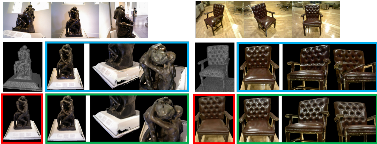
Figure 9: Appearance comparison results for each virtual object used in our paper. The top row shows three example images from original video. The second row are the geometry model and the results from VDTM [4] (in blue rectangle). Note that although VDTM can achieve good visual quality (leftmost), the region of high-fidelity viewpoints is limited. The third row is the fixed texture [21] (in red rectangle) and the results of DOTS (in green rectangle). In contrast to VDTM, DOTS generates omnidirectional synthetic texture maps that produce visually reasonable results.
