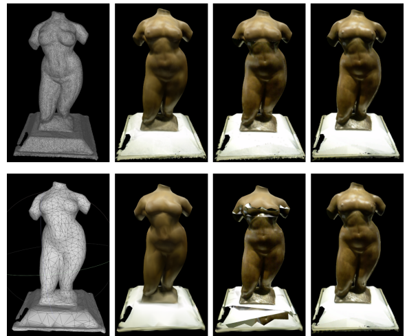
Figure 8: (top) A 3D model rendered using per-vertex color. (bottom) A reduced polygon mesh rendered using a UV map. From left to right: the untextured geometric model, fixed texture mapping [21], VDTM [4], and DOTS.
