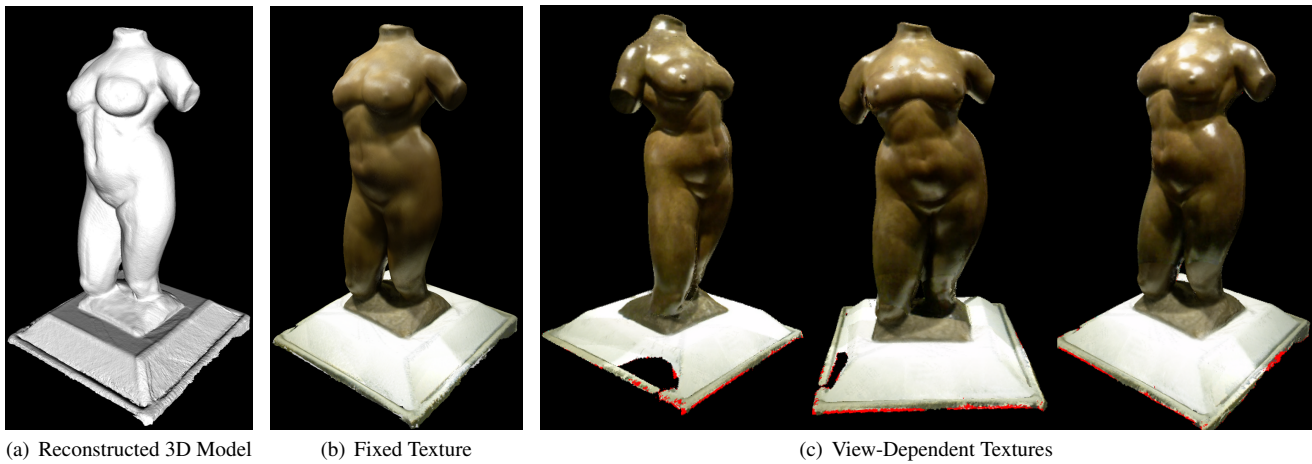
Figure 1: (a) A 3D model reconstructed from images captured with a single consumer depth camera. (b) The textured model generated using the traditional approach of blending color images. (c) Our approach is capable of rendering view-dependent textures in real-time based on the user's head position, thereby providing finer texture detail and better replicating illumination changes and specular reflections that become especially noticeable when observed from different viewpoints in virtual reality.
