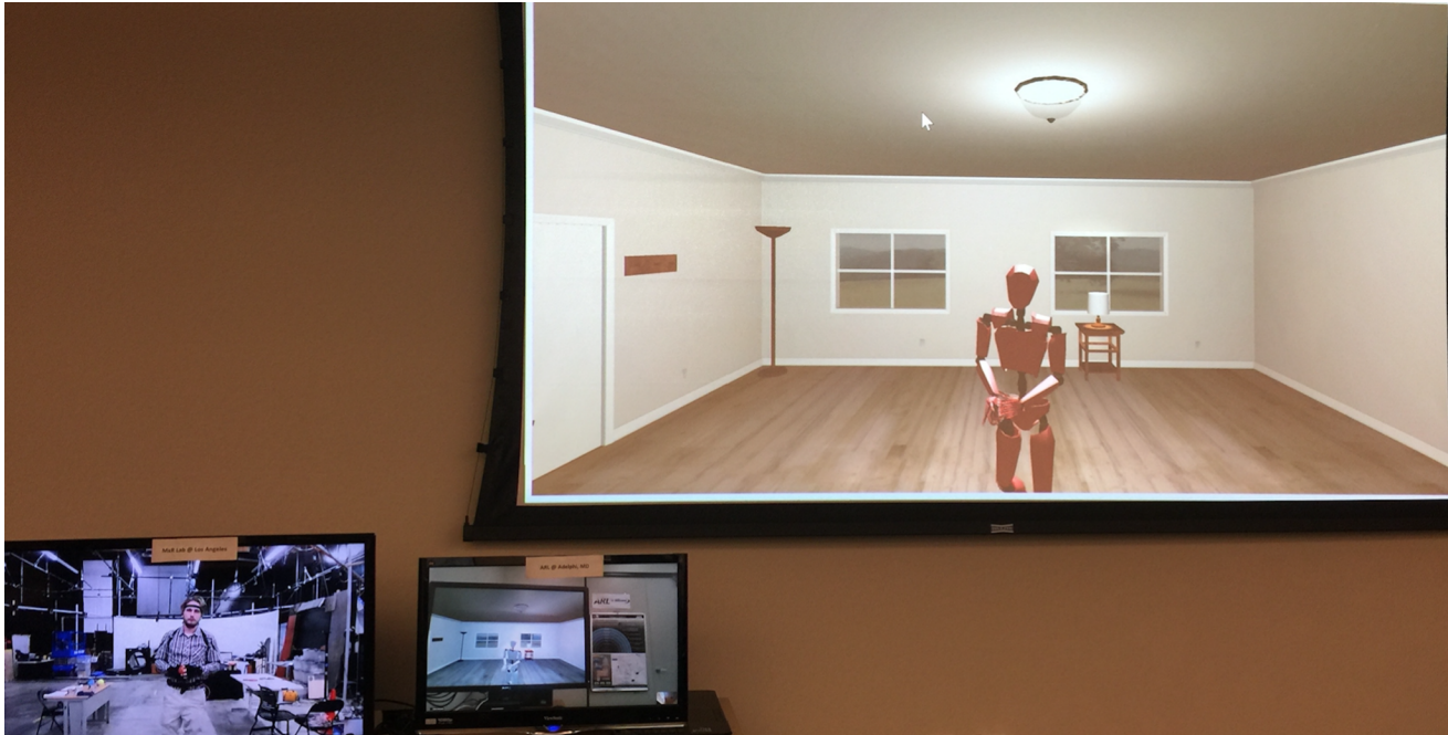
Figure 1: Demo of our system. Bottom left: Remote view of a user in the laboratory’s tracking space. Top right: Local avatar of the user represented in a virtual environment. Bottom center: Video feed of our application running in real time in a remote location.
