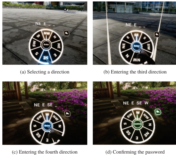
Figure 2: (a) With a current direction of NW , a user presses the SE button on the compass. (b) The user is reoriented towards the SE direction. Note that a glossy frame visualizes the boundary of the scene corresponding to SE after the rotation. The user then presses the enter button to enter SE as the third direction of the password. (c) In the next environment, the user enters W as the last direction in the password. (d) The enter button turns into a confirm button for final confirmation.
