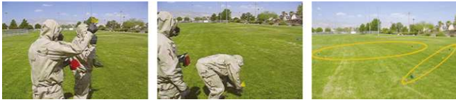
Fig. 1. CST members demonstrate a survey. (Left) The first surveyor signals for a flag and (Center) places it in the ground. (Right) The final flag arrangement with lines circled for emphasis.
