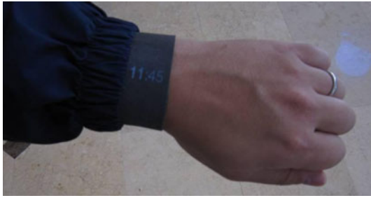
Fig. 11 Low-power projectors mounted in glasses or headsets could illuminate retroreflective clothing for mobile/wearable computing
