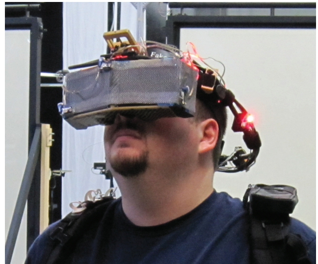
Figure 6: The Wide5 head mounted display provides a horizontal field of view of about 150 degrees. It is used in studies of redirected walking and virtual human interaction.
