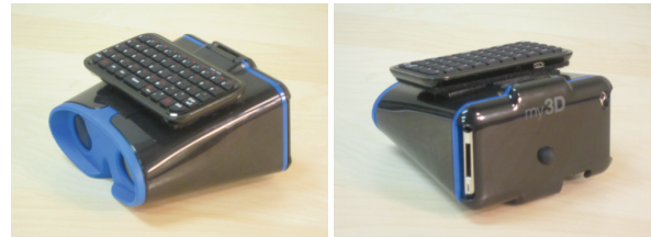
Figure 1: A commodity smartphone based virtual reality system using Hasbro my3D optics.
