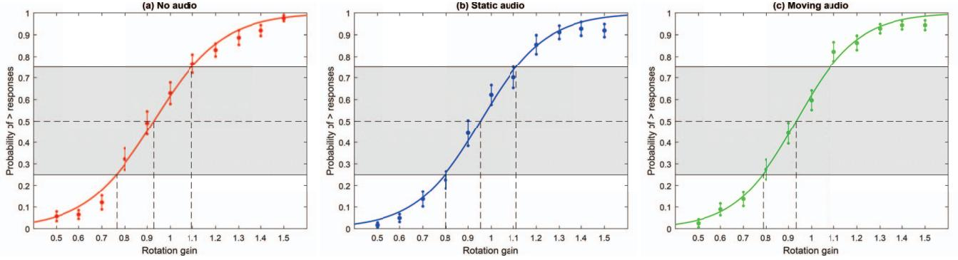
Figure 2: Pooled results of the discrimination between virtual and physical rotation for: (a) no audio, (b) static audio, and (c) moving audio. The x-axes represent the applied rotation gains and the y-axes shows the probability of judging the virtual rotation to be larger than the physical one.
