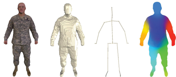
Figure 2: The overview of autorrigging process. Our system first converts the model into the voxel representation to ensure a clean watertight mesh. The control skeleton and skinning weights can then be robustly computed from voxels.
