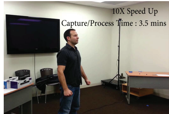
Figure 1: Participants are scanned by rotating their bodies in front of a single Kinect sensor with pauses at four key poses (front, back, and sides). The total scanning time is under a minute.
