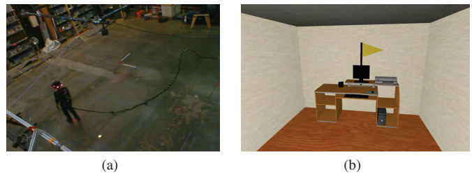
Fig. 3. (a) A user exploring a virtual building while wearing the head-mounted display. (b) A screenshot of the user’s view in the virtual world.
