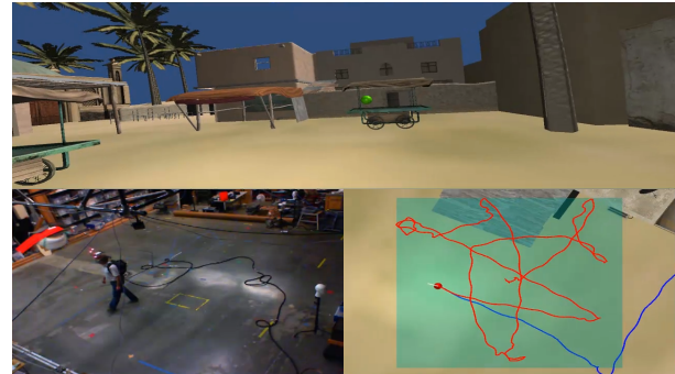
Figure 1: (Bottom) A screenshot of the virtual environment, consisting of a large outdoor scene with multiple buildings to explore. (Bottom Left) The user walking in our lab's motion tracking area while wearing a head-mounted display. (Bottom Right) The user's physical path and virtual path diverge as redirection is applied.
