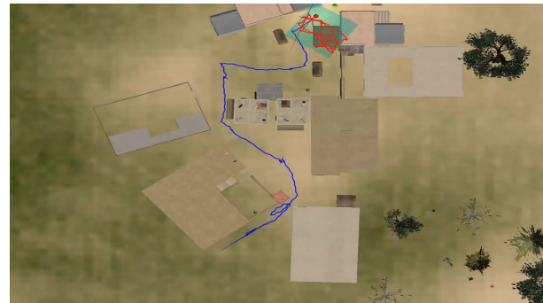
Figure 2: An overhead map of the virtual environment with the user's virtual path indicated in blue. The green rectangle indicates the dimensions of motion capture area with the user's physical walking path overlaid in red.
