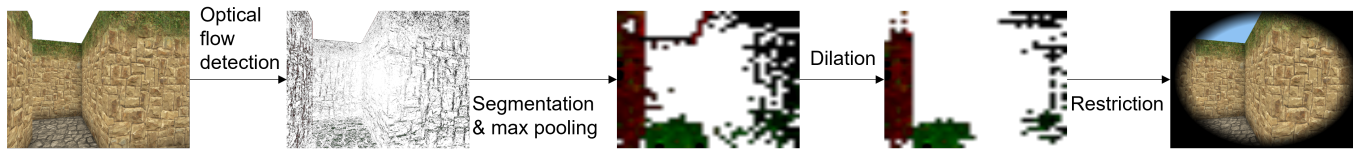
Figure 3: The adaptive field-of-view restrictor is designed as an asymmetric mask that occludes the FOV in high optical-flow regions when the user moves virtually. Based on the image rendered to the screen, per-pixel optical flow is measured in real-time and pooled in a 32 \times 32 grid. Image processing techniques are then used to detect regions of high optical flow and the size and shape of the FOV restrictor is adjusted dynamically.
