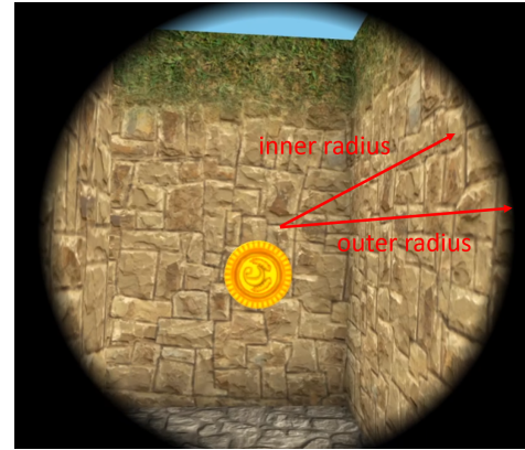
Figure 2: The standard symmetric FOV restriction technique uses a circular black mask to occlude the periphery. The inner and outer radii define the region in which the mask gradually transitions from fully transparent to fully opaque.
