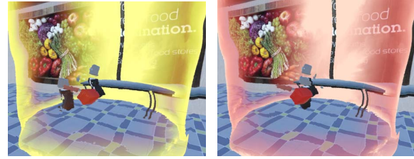
Figure 3: The safe zone is green when the distance between users is greater than six feet. It gradually turns yellow during risky encounters (left) and red when the distance is close to zero (right).
